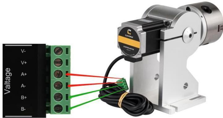
5. Driver takes Cloudray DM542S as an example, adjust the driver dial code, Set current (3.7A) and pulse (12800 or 25600) according to processing requirements (12800: SW1-OFF, SW2-ON, SW3-OFF, SW4-OFF, SW5-ON, SW6-OFF, SW7-OFF, SW8-ON) (25600: SW1-OFF, SW2-ON, SW3-OFF, SW4-OFF, SW5-OFF, SW6-OFF, SW7-OFF, SW8-ON)
