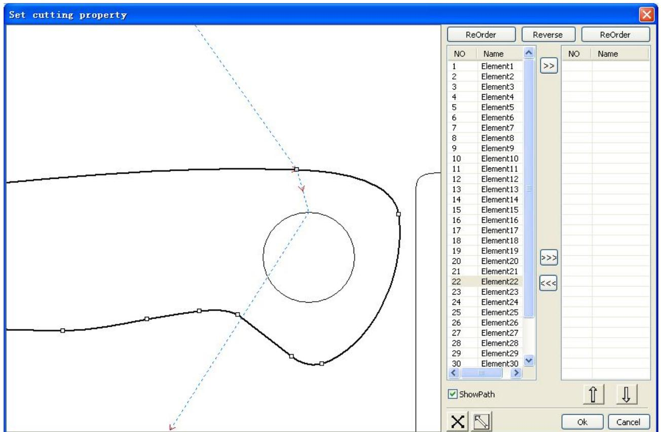
Select the graphics that should be changed the cutting point, it will show all the nodes in the current graphics. Select the starting point, double-click the mouse, it will change the starting point of the current graphics. After the completion of all changes, click
