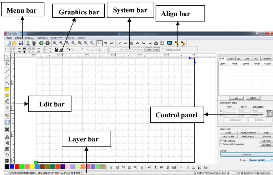
**Menu Bar:** The main function of this software are available through the implementation of the Menu Bar. Execute the menu command is the most basic mode of operation. Menu Bar including: Document、 Edit、 Draw、 Setting、 Processing、 View and Help.
