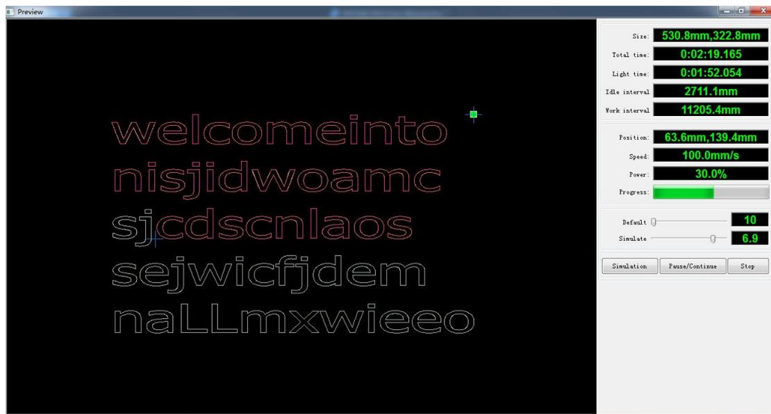
Software supports the preview of the documents to be processed, and you can get some basic information through the preview. For example, the path of the actual output of the processing, general processing time, processing the distance. The machining process can be simulated.
